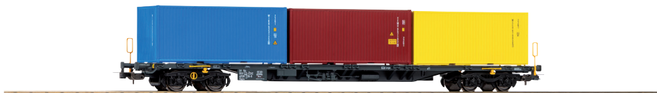
24634 Flat car w container Sgnss ČD VI, loaded with 3 containers
